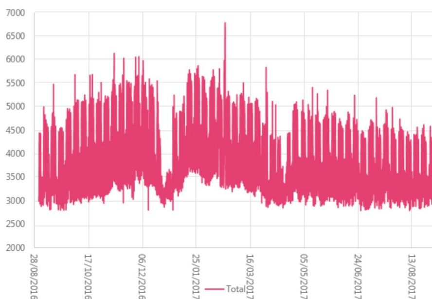
Figure 15 Measured Yearly Campus Electrical Demand in kW.
